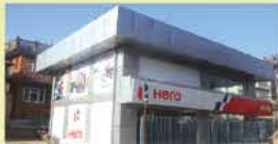
Bike Showroom At Chabahil Made Up Of (Double Storey) MS Steel Structure With Prefab Panel.
